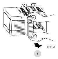
Slide module out of chassis.
