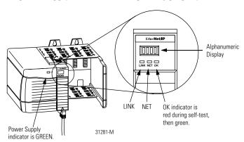
The alphanumeric display should cycle through the following states: "TEST - PASS - OK - REV x.x," where "x.x" is the module's firmware revision. The display then alternates between "OK" and the module's EtherNet/IP address.
