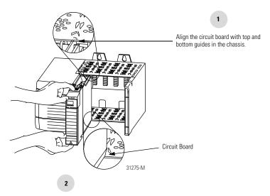
Slide the module into the chassis. Make sure the module backplane connector properly connects to the chassis backplane.
