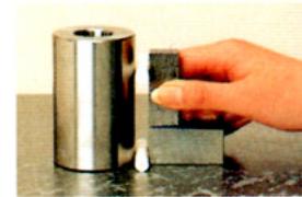
Checking right angle
