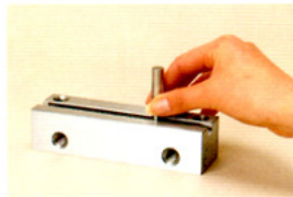
Measuring width of groove
