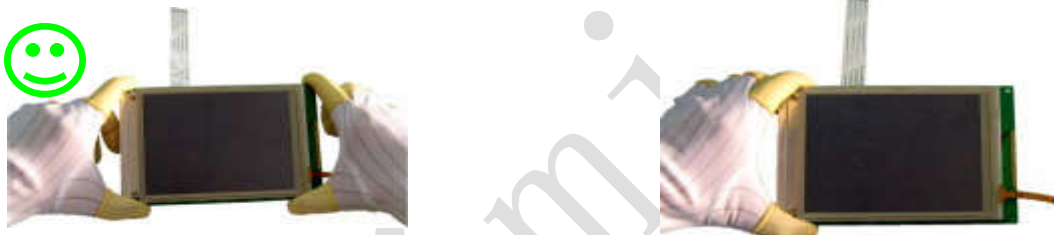
As above picture, please handle with anti-static gloves around LCM edges.
