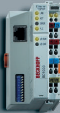
Bus Terminal Controller series BC with integrated IEC 61131-3 PLC
